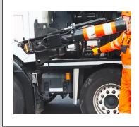
Swing-up stabiliser rotating away from Operator on opposite side of vehicle (manufacturer dependent)
