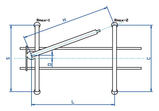
S = Span of loader crane stabilisers, m
